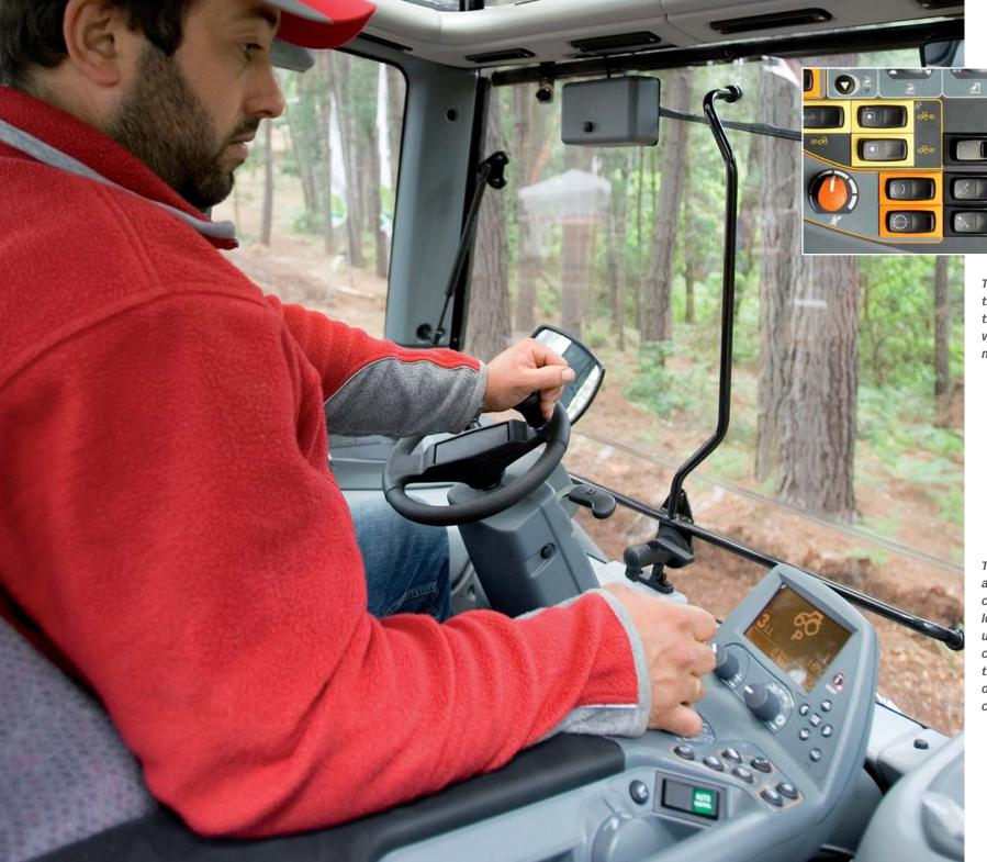
The new design and positioning of the switches on the side panels combined with the use of colour coding makes them easy to use.
