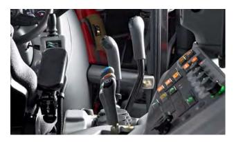
Mechanical or electronically controlled ancillary hydraulics can be specified as required, and control is straightforward and logical. Long hydraulic oil change intervals save time and costs. The T Series allows for the optional use of Valtra-approved bio oils.
