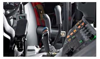
The N Series lets you choose between mechanical or electronically controlled hydraulics. Controlling the hydraulics is straightforward and logical. The hydraulic oil change interval is 2000 hours, which saves time and costs. The N Series also allows for the optional use of bio-oils.
