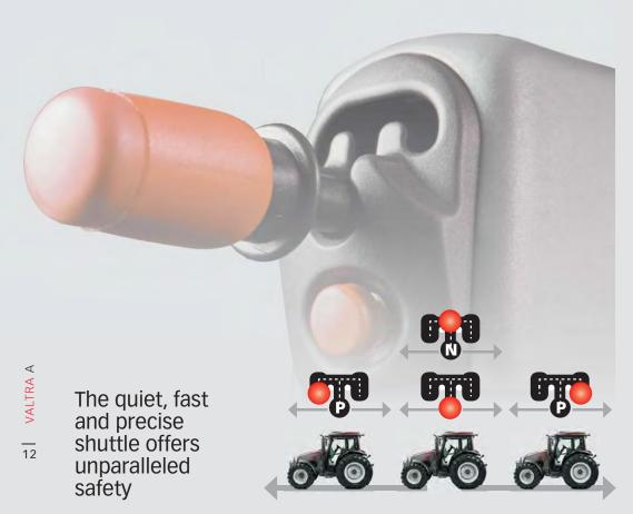
Valtra HiTech tractors combine car comfort, excellent features and simple joystick control. You only have to give the orders, which you can do with a light touch of the fingertips. Each HiTech tractor is an individual machine whose behaviour can be modified to your liking. HiTech tractors are comfortable, efficient, easy to operate and safe.
