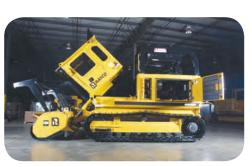
Hydraulic Tilt Cab For Easy Access to Engine and Hydraulic Components
