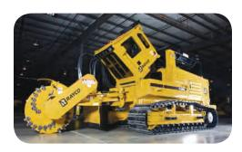
Tilt Cab for Access to Hydraulic Components
