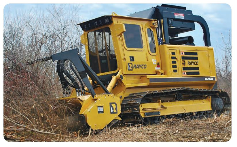
Rayco's C260 Crawler is a mid-sized mulcher that delivers 260 hp in a compact, low ground pressure package. A powerful Cummins QSB6.7L turbo diesel engine powers the C260. Rayco's exclusive elevated cooling design keeps engine and hydraulic temperatures within their limits in the harshest of environments. A reversing fan can be activated from the cab to clear the limbriser debris screens.
