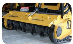
Predator Mulcher Head with Variable Displacement Motor
