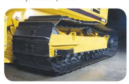
Heavy Duty Undercarriage with 2-Speed Final Drives
