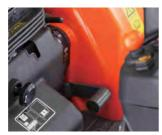
**Parking Brake** A buzzer sounds if the operator leaves the seat without setting the parking brake.
