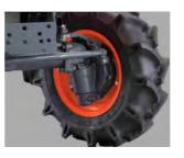
**Bevel-Gear 4WD** When the going gets tough, the new B1 Series keeps going, thanks to a bevelgear 4WD that provides power to all four wheels whenever extra traction is required. Bevel-gear 4WD also provides a higher ground clearance as well as the tightest turning radius in the new B1 Series' class.
