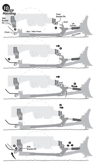
▲ Important: There should be a gap (3/8" or larger) Bracket I between the inside of the hook to the front of the bracket pin. The amount of gap may vary between specific models, but having a gap at this location is important.
