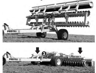
E. Place both the Transport Cylinders (#3) and the Wing Cylinders (#2) into the FLOAT position before operation.
