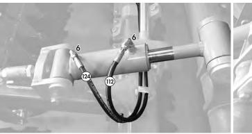
Detail B - LH Wheel Cylinder Configuration (RH is Opposite)
