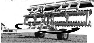
D. After fully opening the wings, extend the Transport Cylinders (#3) to completely lower the Pro-Till rear frame sections to the ground.
