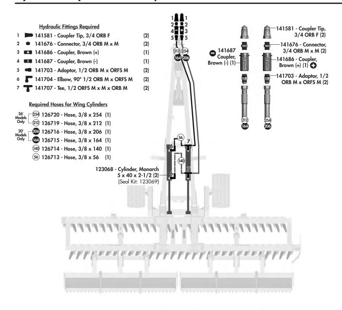
Transport Cylinder Hose Connection Detail
