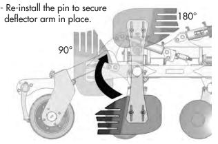
If preferred, the deflector arm could also be completely removed and stored by pulling the pin and removing.
