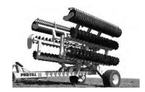
D. When the wings get close to the wing transport holders, you may need to *slightly* extend the Transport cylinders (#3) so the rollers can reach the correct position.
