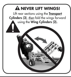
C. After raising all the rear sections, retract the Wing cylinders (#2) to bring both wings inward towards the frame.
