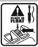
**IMPORTANT:** The Transport Cylinders and Wing Cylinders **MUST** both be in the **FLOAT**
