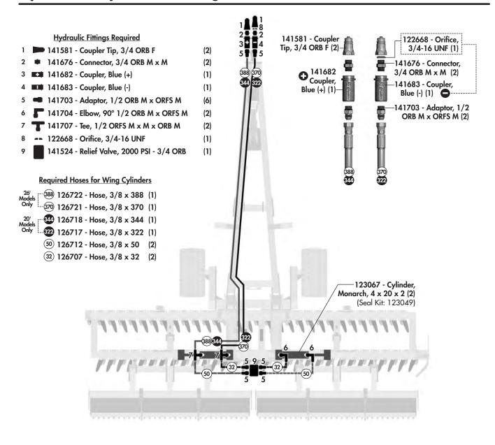
**Relief Valve Connections Detail**
