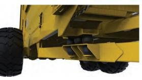
Tandem walking wheels cut uneven terrain in half with a massive unrestricted range of motion. All four wheels are always in contact with the ground surface. Coupled with a wide stance, these machines will ride over the roughest terrain with ease and control.
