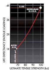
of standard grade A36, resists rust and shock loading better. As a result, the cutter lasts longer, endures more
