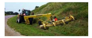
unit is going in. The two vertical cross-joints also absorb any misalignment or deviation from 90 degrees. These extras mean the Sidearm® goes farther, lasts longer and can take on practically anything put in its path.
