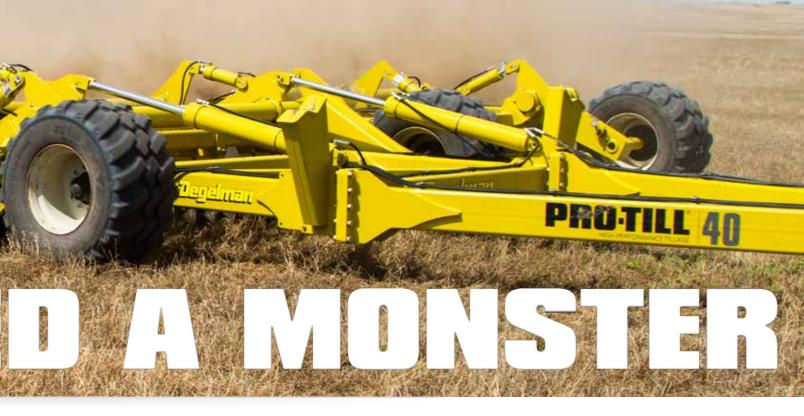
Pro-Till® is ideally pulled fast - 10 to 14 mph fast. Our patent pending combination of independent disc arms, with small diameter shallow discs, motion dampening rubber suspension, sturdy frame and cutting edge consolidating rollers allow this tillage tool to slice through residue as never seen before. Pro-Till® will cut, weed, throw and mix soils at incredible speeds and usually in one pass. This is a true residue-killing machine.
