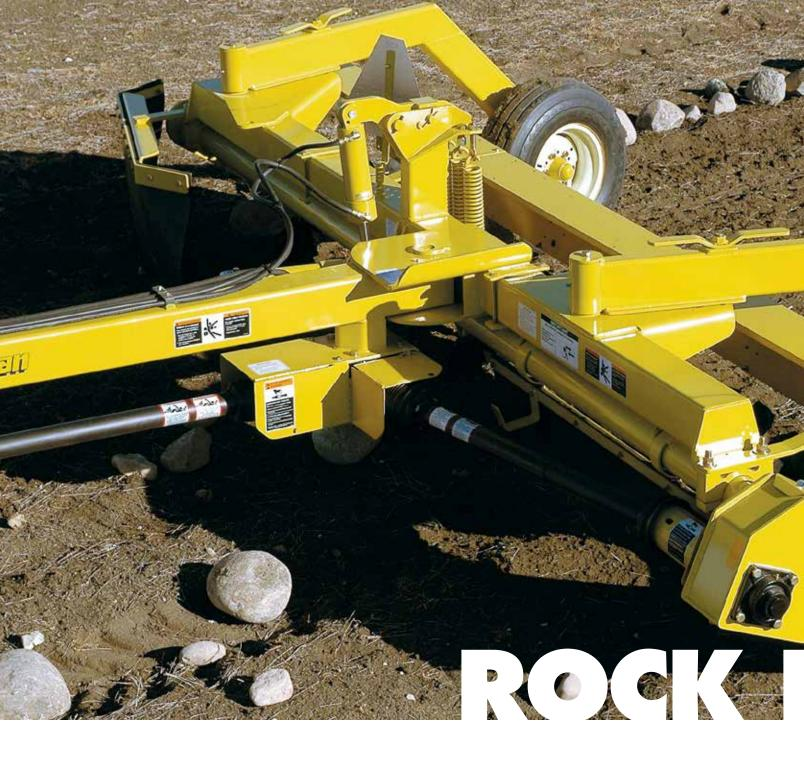
Built in the Degelman tradition of quality rock removal equipment, the RR1500 Rock Rake tackles a variety of jobs, including windrowing rocks for subsequent picking, reclaiming gravel on secondary roads, conditioning soil for the construction of golf courses, and leaving a well-groomed final finish for optimum seeding.
